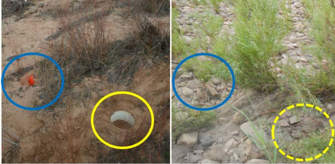
Figure 26. Slickrock Downstream sediment trap and erosion stake; pre-release photo on left (3/22/17), and post-release photo on right (7/6/17). Note the scouring of fine material observed with the orange erosion stake circled in blue between pre- and post-release. It appears that strong flows ripped out sediment trap pre- versus post-release.
