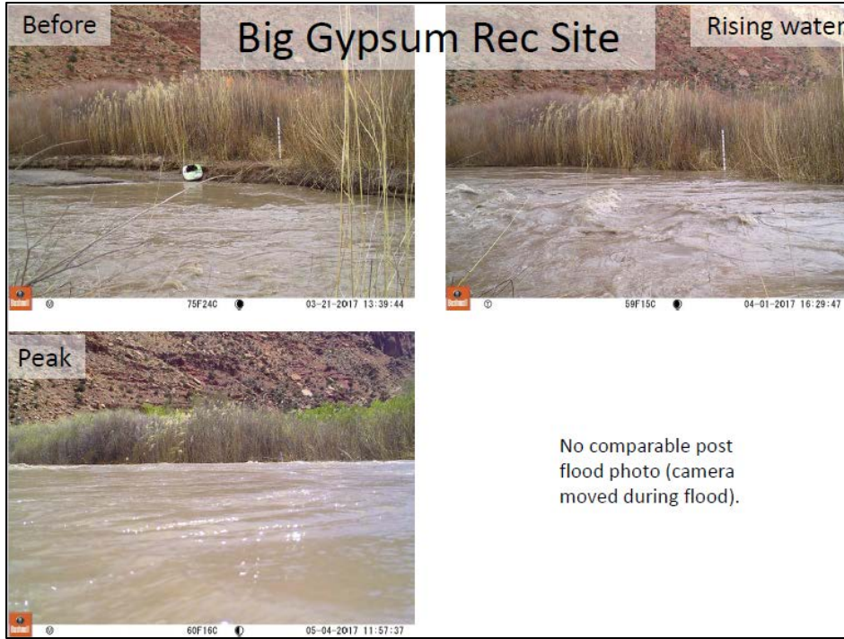
Figure 46. BLM Rec (Big Gypsum) staff gage at pre-release, rising water, and peak-release.
