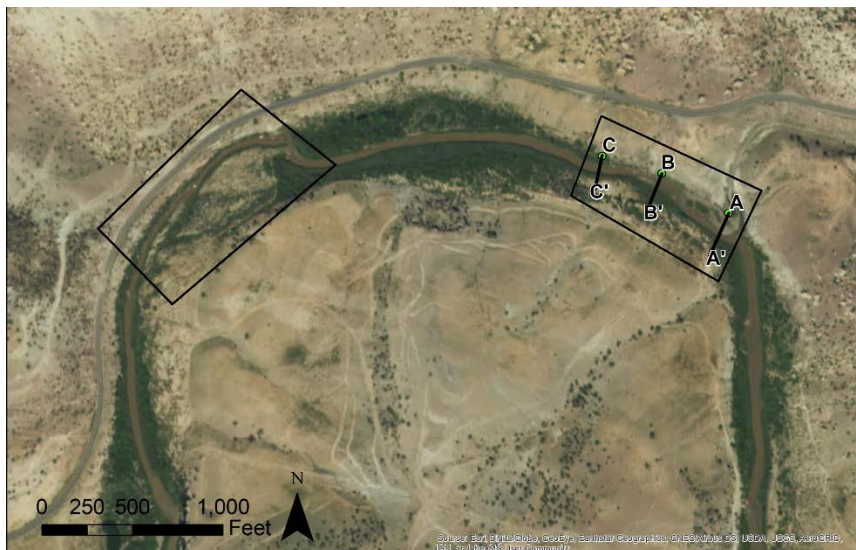
Figure 41. The Slickrock Downstream site (left) and the Fort Lewis College site farther upstream showing cross-sections analyzed with structure from motion technology.
